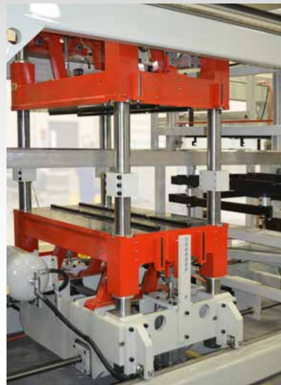
Independent top and bottom servo plug drives for better material distribution
