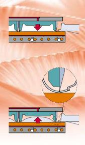
**Heating** - Plastic material is unwound from a roll and fed into the forming area. Here it is trapped in place by a double toggle mechanism which closes the forming press. Compressed air is injected through the mould ensuring complete contact of the plastic material with the heating platen. Exact, uniform and rapid heating is achieved by the unique heating platen assembly.
