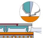
**Cutting** - As the forming air is vented, a second toggle movement forces the knife edge of the cutting die through the plastic sheet.
